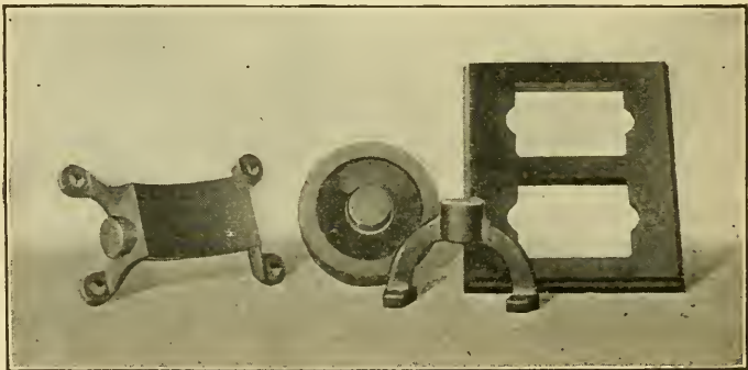
Fig. 271A—Several ordinary patterns without core prints
